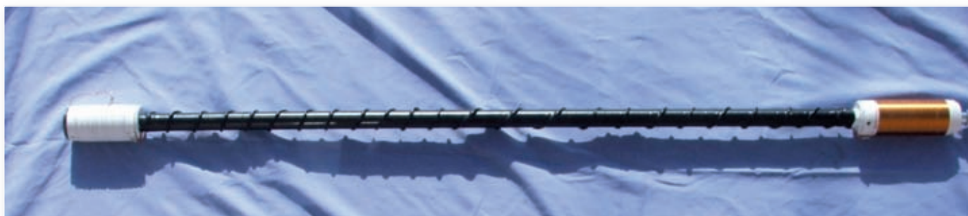
Fig. 4: The final assembly is firmly fixed using epoxy resin or similar adhesive.
