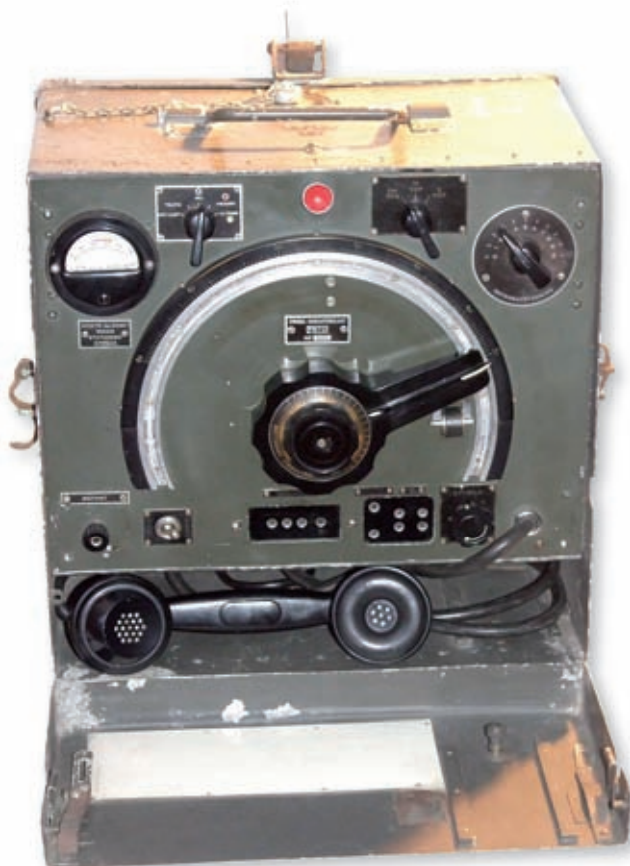
Fig. 1: The Swedish transmitter receiver with large tuning dial.
