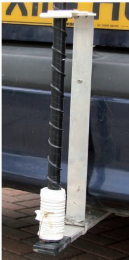
Fig. 5: The final tuning must be done while the antenna is mounted on the vehicle to be used. Chris G4DCH recommends using a suitable antenna analyser.
