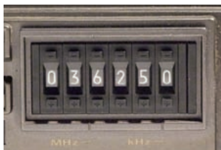
Fig. 4: The Frequency selection switches with mechanical up/down buttons.
