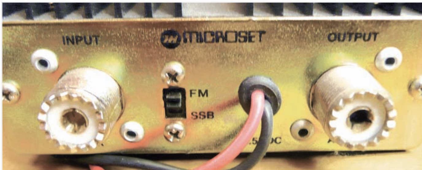
Fig. 1: The Microset 144MHz amplifier has a two position switch that allows different 'hang-times' to be set for its r.f. sensing switch-over circuitry. The short time is suitable for f.m. work, but a longer delay is more suitable for s.s.b. activity, when there's only an output when speaking.
