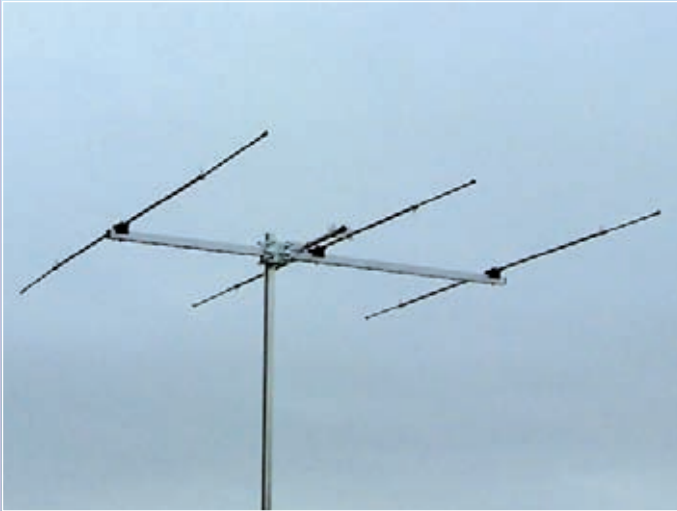
Fig. 1: The Moonraker YG3 4 70MHz 3-element Yagi antenna. The slightly thinner looking outer elements are telescopic, and slide into the main elements. This was the feature that first attracted G3XFD's attention, for ease of assembly for portable operations.
